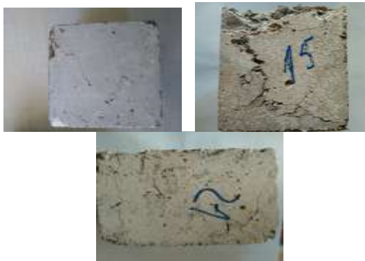
Figure 5 : Samples after heat expose in 200 0 C, 400 0 C and 600 0 C
