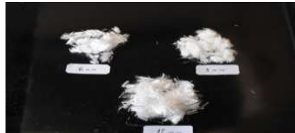
Figure 2: Polypropylene fibers 12 mm (PP1); 6 mm (PP2); 3 mm (PP3)
