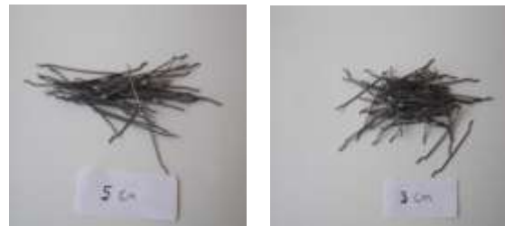
Figure1: Steel Fiber 5 cm in length (SF1) and steel fiber 3 cm in length (SF2)
